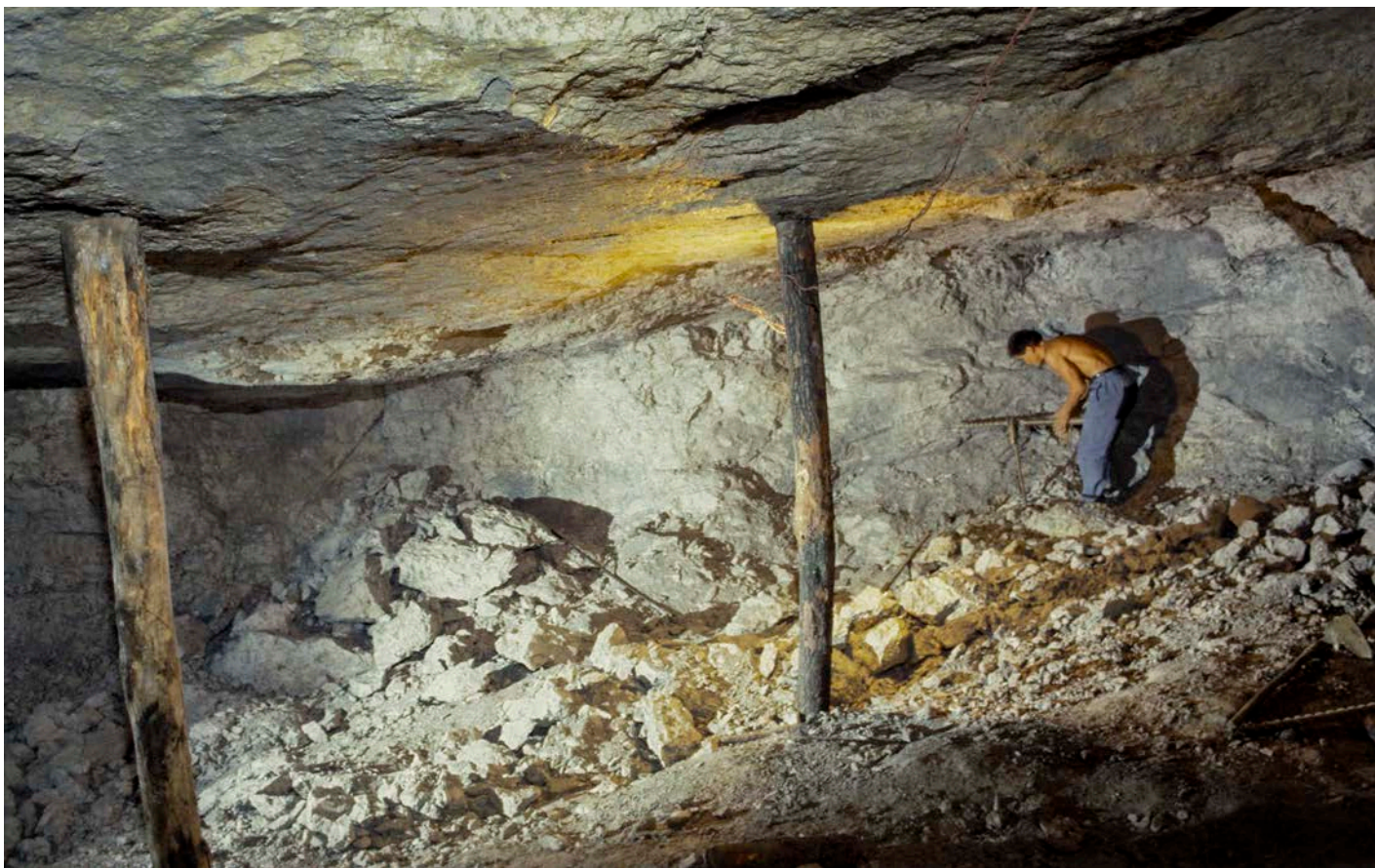
Pyrite and sulphur production at Xingwen, China. Top. A room in a small pyrite mine near Xingwen. The miner is drilling a new shothole to widen the room, while props are already installed under loose sections of the roof. Bottom left. A young lad drags a skid-mounted basket of coal out of the mine that he works with his brother near Xingyan. Bottom right. One of the lines of 20 furnaces at the Xingyan sulphur factory, at Xingwen, China, with limestone hills across the skyline. The arched roofs are on the condensation rooms just to the right of their matching furnaces. Some of the roof holes on the furnaces are open for recharging, whereas others are sealed during firing.
