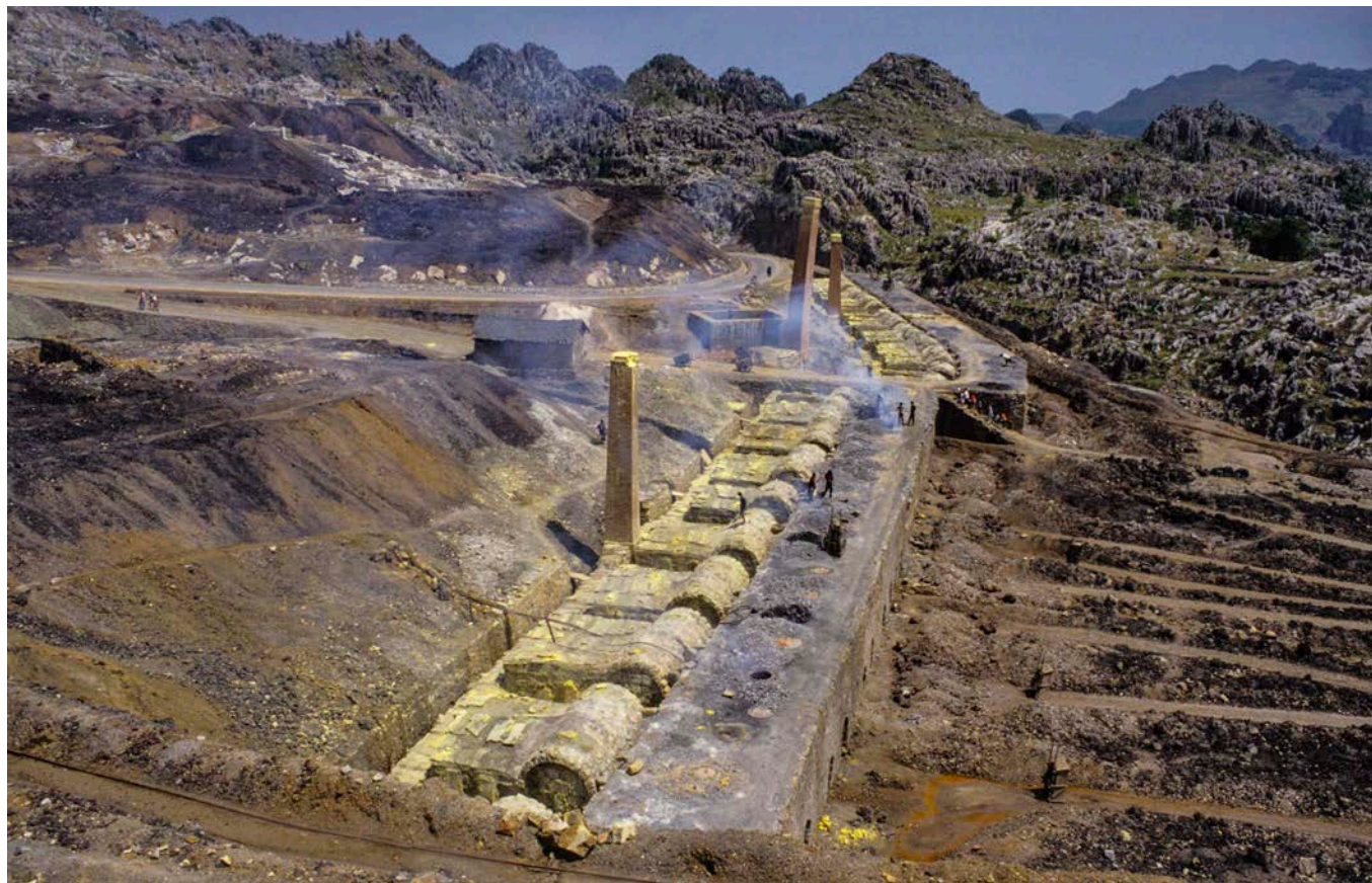
Plate 6. Waste heaps spread-out on each side of the Xingyan sulphur furnaces. Tip heaps on the left are sub-grade ore and also waste from an older generation of furnaces higher up the slope. Debris on the right is the top end only of the great piles of slag raked-out from each furnace after each firing. Downslope drainage takes contaminated water on to the limestone towards the right. The prevailing wind is to the left and air pollution restricts plant growth on the higher slopes.
