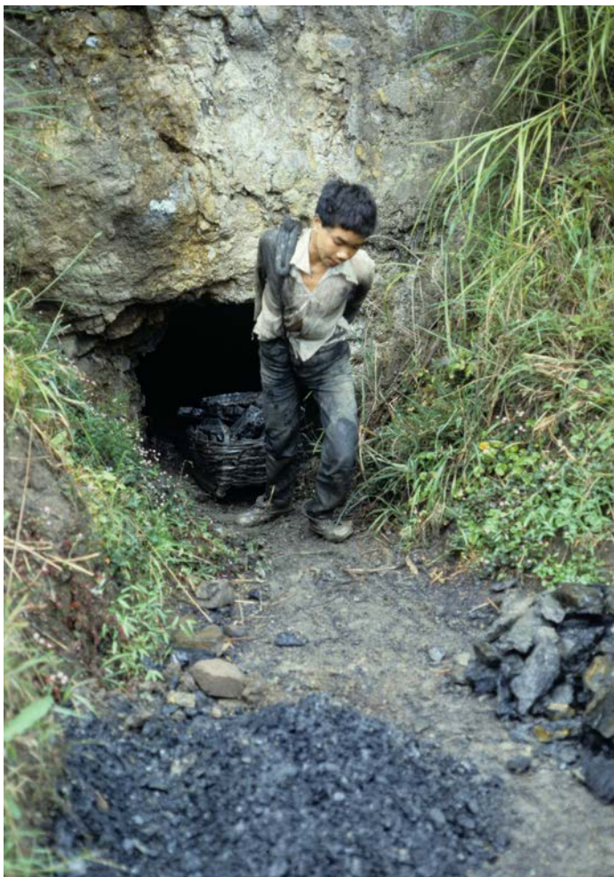
Pyrite and sulphur production at Xingwen, China. Top. A room in a small pyrite mine near Xingwen. The miner is drilling a new shothole to widen the room, while props are already installed under loose sections of the roof. Bottom left. A young lad drags a skid-mounted basket of coal out of the mine that he works with his brother near Xingyan. Bottom right. One of the lines of 20 furnaces at the Xingyan sulphur factory, at Xingwen, China, with limestone hills across the skyline. The arched roofs are on the condensation rooms just to the right of their matching furnaces. Some of the roof holes on the furnaces are open for recharging, whereas others are sealed during firing.
