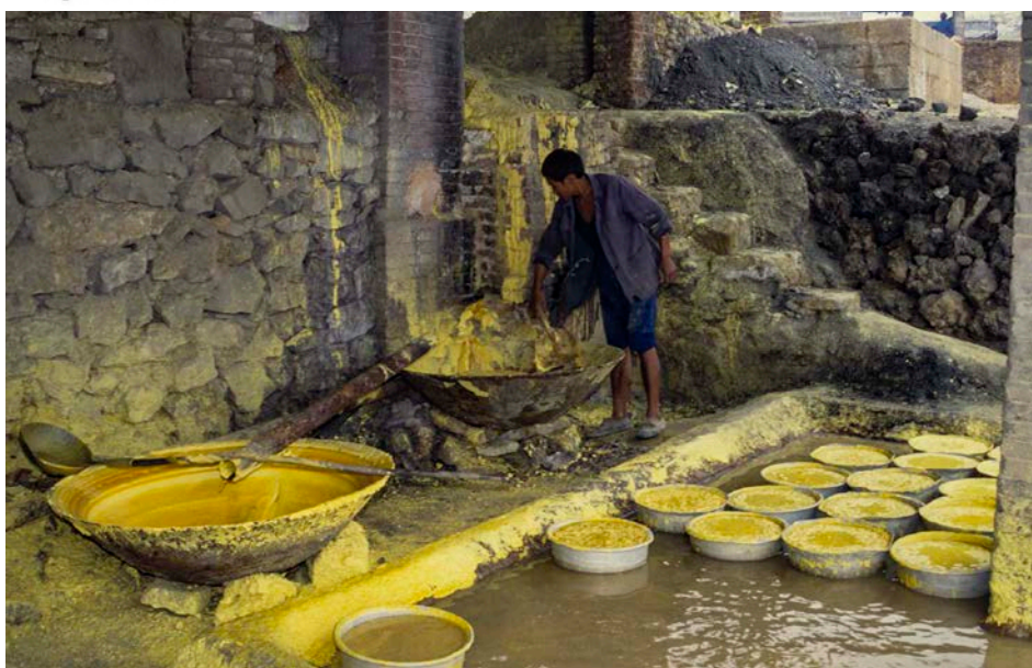
Plate 5 (below). Molten sulphur has been poured through the vats to fill the cooled bowls in the final production stage at the Xingyan sulphur factory.
