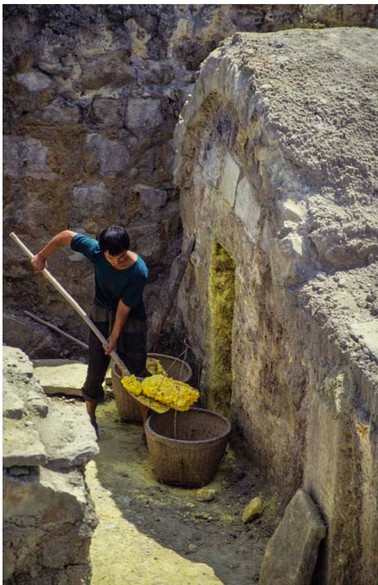
Plate 4 (above). Blocks of sulphur are shovelled out of a cooled condensation room adjacent to its furnace in the Xingyan sulphur factory.
