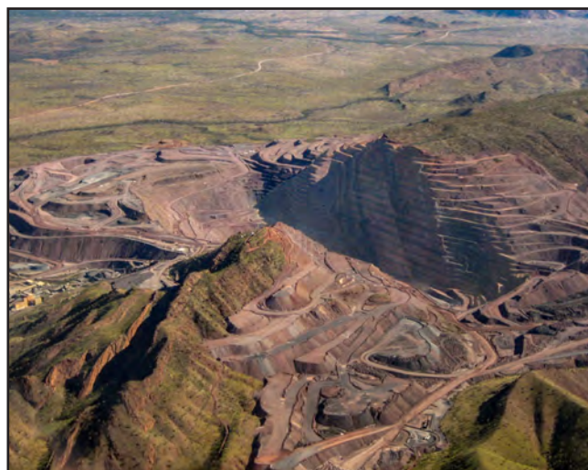
Figure 10. The open pit of the Argyle diamond mine, in Western Australia, which had evolved into underground working in 2013.
