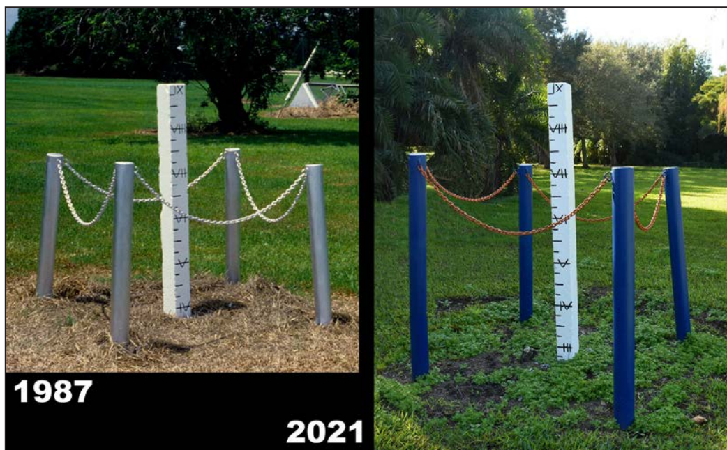
Figure 3. Comparative images of the Subsidence Post at Belle Glade in the Florida Everglades in 1987 and 2021. Posts for the chain fence also reach down to bedrock beneath the peat. The post now has an explanatory signboard, which was temporarily removed to take the later photograph.
